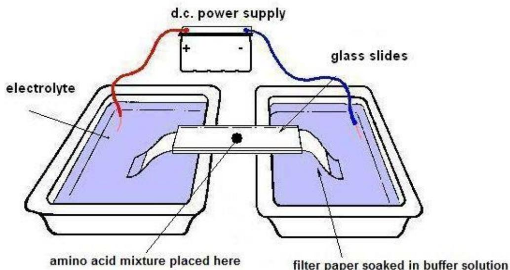
Marks: power supply / electrolyte + filter paper / buffer / acid mixture central
