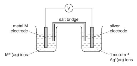
The metal electrodes of the two half-cells were connected via a voltmeter, reading to two decimal places. This was used to measure the cell potential of the cell.
