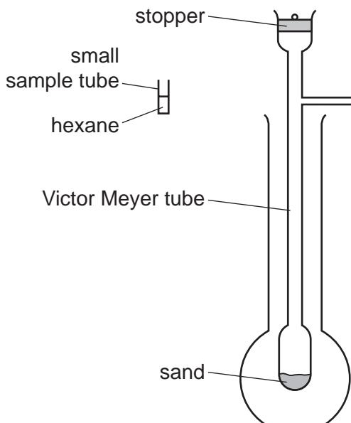
A small sample tube containing the hexane is inserted at the top of the Victor Meyer tube. The sample tube is small enough to fit inside the Victor Meyer tube and falls freely onto the hot sand below. The sand will cushion its fall so that the sample tube does not break. The stopper is then quickly replaced at the top of the Victor Meyer tube. The hot sand causes the hexane to vaporise and expel air contained in the Victor Meyer tube.
