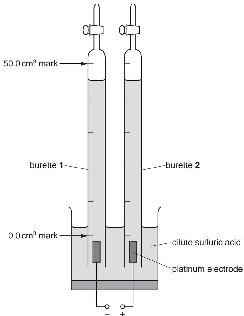
reaction at electrode in burette 1:  $2\text{H}^+(\text{aq}) + 2\text{e}^- \rightarrow \text{H}_2(\text{g})$
