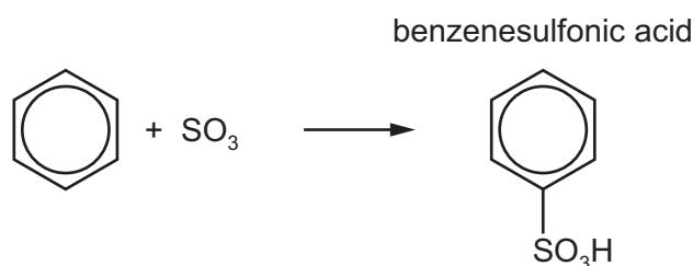
The mechanism of this reaction is similar to that of the nitration of benzene. Concentrated  $\text{H}_2\text{SO}_4$  is used in an initial step to generate the  $\text{SO}_3\text{H}^+$  electrophile as shown.
