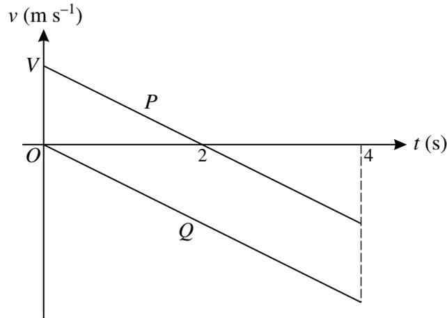
Two particles  $P$  and  $Q$  move vertically under gravity. The graphs show the upward velocity  $v \text{ m s}^{-1}$  of the particles at time  $t \text{ s}$ , for  $0 \leq t \leq 4$ .  $P$  starts with velocity  $V \text{ m s}^{-1}$  and  $Q$  starts from rest.
