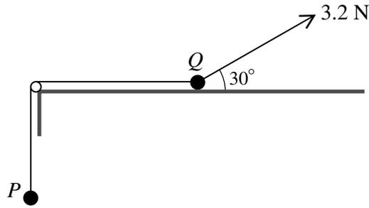
Particles  $P$  and  $Q$ , of masses  $0.2\text{ kg}$  and  $0.5\text{ kg}$  respectively, are connected by a light inextensible string. The string passes over a smooth pulley at the edge of a rough horizontal table.  $P$  hangs freely and  $Q$  is in contact with the table. A force of magnitude  $3.2\text{ N}$  acts on  $Q$ , upwards and away from the pulley, at an angle of  $30^\circ$  to the horizontal (see diagram).
