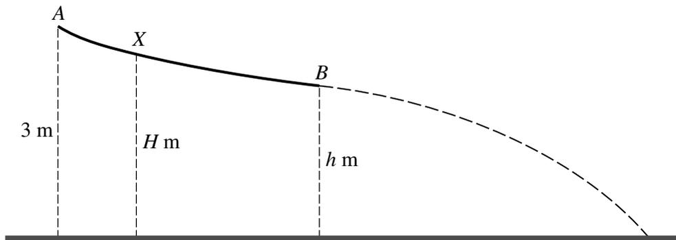
A smooth slide  $AB$  is fixed so that its highest point  $A$  is  $3 \text{ m}$  above horizontal ground.  $B$  is  $h \text{ m}$  above the ground. A particle  $P$  of mass  $0.2 \text{ kg}$  is released from rest at a point on the slide. The particle moves down the slide and, after passing  $B$ , continues moving until it hits the ground (see diagram). The speed of  $P$  at  $B$  is  $v_B$  and the speed at which  $P$  hits the ground is  $v_G$ .
