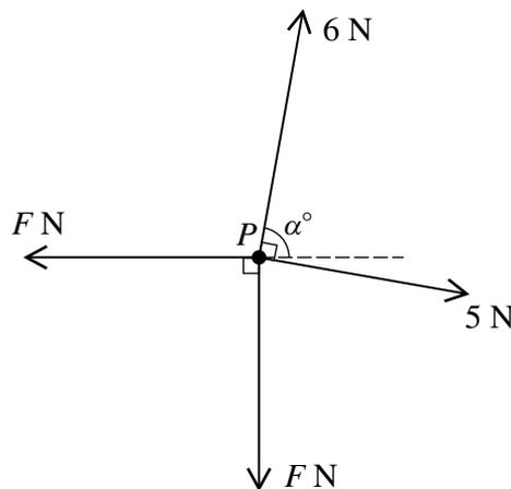
A particle  $P$  is in equilibrium on a smooth horizontal table under the action of four horizontal forces of magnitudes 6 N, 5 N,  $F$  N and  $F$  N acting in the directions shown. Find the values of  $\alpha$  and  $F$ . [6]
