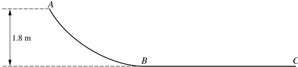
The diagram shows the vertical cross-section  $ABC$  of a fixed surface.  $AB$  is a curve and  $BC$  is a horizontal straight line. The part of the surface containing  $AB$  is smooth and the part containing  $BC$  is rough.  $A$  is at a height of 1.8 m above  $BC$ . A particle of mass 0.5 kg is released from rest at  $A$  and travels along the surface to  $C$ .
