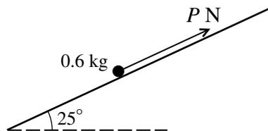
The diagram shows a particle of mass 0.6 kg on a plane inclined at  $25^\circ$  to the horizontal. The particle is acted on by a force of magnitude  $P \text{ N}$  directed up the plane parallel to a line of greatest slope. The coefficient of friction between the particle and the plane is 0.36. Given that the particle is in equilibrium, find the set of possible values of  $P$ . [9]
