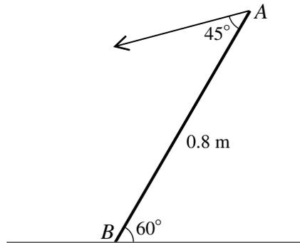
A uniform rod  $AB$  has weight  $6 \text{ N}$  and length  $0.8 \text{ m}$ . The rod rests in limiting equilibrium with  $B$  in contact with a rough horizontal surface and  $AB$  inclined at  $60^\circ$  to the horizontal. Equilibrium is maintained by a force, in the vertical plane containing  $AB$ , acting at  $A$  at an angle of  $45^\circ$  to  $AB$  (see diagram). Calculate
