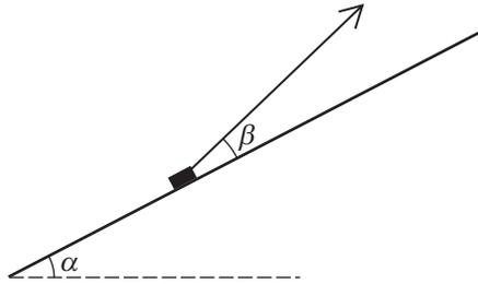
A small block of weight 5.1 N rests on a smooth plane inclined at an angle  $\alpha$  to the horizontal, where  $\sin \alpha = \frac{8}{17}$ . The block is held in equilibrium by means of a light inextensible string. The string makes an angle  $\beta$  above the line of greatest slope on which the block rests, where  $\sin \beta = \frac{7}{25}$  (see diagram). Find the tension in the string. [3]
