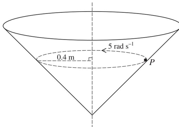
A particle  $P$  of mass  $0.5 \text{ kg}$  moves in a horizontal circle on the smooth inner surface of a hollow cone which is fixed with its axis vertical and its vertex downwards.  $P$  moves with angular speed  $5 \text{ rad s}^{-1}$  in a circle of radius  $0.4 \text{ m}$  (see diagram). Show that the semi-vertical angle of the cone is  $45^\circ$  and calculate the magnitude of the force exerted on  $P$  by the surface of the cone. [6]
