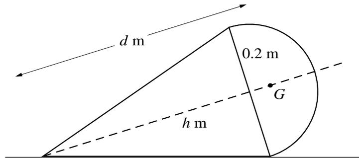
An object is formed by joining a hemispherical shell of radius 0.2 m and a solid cone with base radius 0.2 m and height  $h$  m along their circumferences. The centre of mass,  $G$ , of the object is  $d$  m from the vertex of the cone on the axis of symmetry of the object. The object rests in equilibrium on a horizontal plane, with the curved surface of the cone in contact with the plane (see diagram). The object is on the point of toppling.
