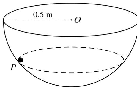
A particle  $P$  of mass  $0.4 \text{ kg}$  moves with constant speed in a horizontal circle on the smooth inner surface of a fixed hollow hemisphere with centre  $O$  and radius  $0.5 \text{ m}$  (see diagram).
