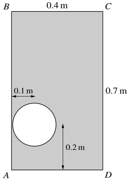
A uniform object is made by drilling a cylindrical hole through a rectangular block. The axis of the cylindrical hole is perpendicular to the cross-section  $ABCD$  through the centre of mass of the object.  $AB = CD = 0.7$  m,  $BC = AD = 0.4$  m, and the centre of the hole is 0.1 m from  $AB$  and 0.2 m from  $AD$  (see diagram). The hole has a cross-section of area  $0.03$  m<sup>2</sup>.
