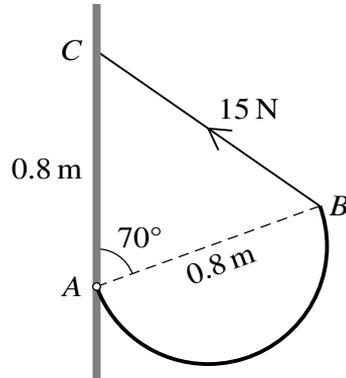
A uniform wire has the shape of a semicircular arc, with diameter  $AB$  of length  $0.8 \text{ m}$ . The wire is attached to a vertical wall by a smooth hinge at  $A$ . The wire is held in equilibrium with  $AB$  inclined at  $70^\circ$  to the upward vertical by a light string attached to  $B$ . The other end of the string is attached to the point  $C$  on the wall  $0.8 \text{ m}$  vertically above  $A$ . The tension in the string is  $15 \text{ N}$  (see diagram).
