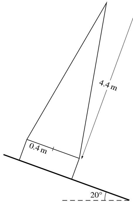
A uniform solid cone has base radius 0.4 m and height 4.4 m. A uniform solid cylinder has radius 0.4 m and weight equal to the weight of the cone. An object is formed by attaching the cylinder to the cone so that the base of the cone and a circular face of the cylinder are in contact and their circumferences coincide. The object rests in equilibrium with its circular base on a plane inclined at an angle of  $20^\circ$  to the horizontal (see diagram).
