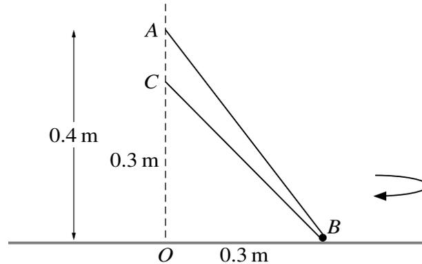
A light inextensible string passes through a small smooth bead  $B$  of mass  $0.4\text{ kg}$ . One end of the string is attached to a fixed point  $A$   $0.4\text{ m}$  above a fixed point  $O$  on a smooth horizontal surface. The other end of the string is attached to a fixed point  $C$  which is vertically below  $A$  and  $0.3\text{ m}$  above the surface. The bead moves with constant speed on the surface in a circle with centre  $O$  and radius  $0.3\text{ m}$  (see diagram).
