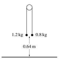
Two particles of masses  $1.2\,\mathrm{kg}$  and  $0.8\,\mathrm{kg}$  are connected by a light inextensible string that passes over a fixed smooth pulley. The particles hang vertically. The system is released from rest with both particles  $0.64\,\mathrm{m}$  above the floor (see diagram). In the subsequent motion the  $0.8\,\mathrm{kg}$  particle does not reach the pulley.
