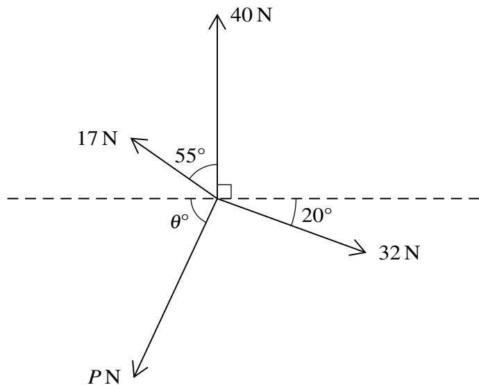
Coplanar forces of magnitudes 40 N, 32 N,  $P$  N and 17 N act at a point in the directions shown in the diagram. The system is in equilibrium. Find the values of  $P$  and  $\theta$ . [6]
