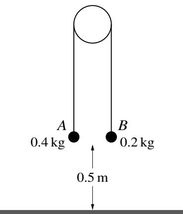
Two particles  $A$  and  $B$ , of masses 0.4 kg and 0.2 kg respectively, are connected by a light inextensible string which passes over a fixed smooth pulley. Both  $A$  and  $B$  are 0.5 m above the ground. The particles hang vertically (see diagram). The particles are released from rest. In the subsequent motion  $B$  does not reach the pulley and  $A$  remains at rest after reaching the ground.
