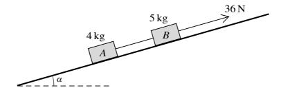
Two blocks A and B of masses 4 kg and 5 kg respectively are joined by a light inextensible string. The blocks rest on a smooth plane inclined at an angle  $\alpha$  to the horizontal, where  $\tan \alpha = \frac{7}{24}$ . The string is parallel to a line of greatest slope of the plane with B above A. A force of magnitude 36 N acts on B, parallel to a line of greatest slope of the plane (see diagram).
