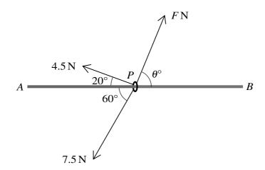
A small ring P is threaded on a fixed smooth horizontal rod AB. Three horizontal forces of magnitudes 4.5 N, 7.5 N and F N act on P (see diagram).
