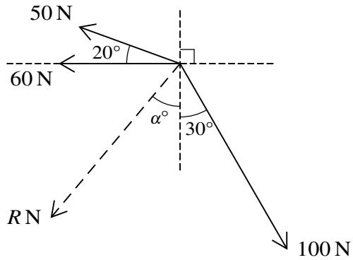
Three coplanar forces of magnitudes 50 N, 60 N and 100 N act at a point. The resultant of the forces has magnitude  $R$  N. The directions of these forces are shown in the diagram. Find the values of  $R$  and  $\alpha$ . [6]
