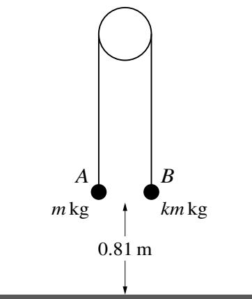
Two particles  $A$  and  $B$  have masses  $m$  kg and  $km$  kg respectively, where  $k > 1$ . The particles are attached to the ends of a light inextensible string. The string passes over a fixed smooth pulley and the particles hang vertically below it. Both particles are at a height of 0.81 m above horizontal ground (see diagram). The system is released from rest and particle  $B$  reaches the ground 0.9 s later. The particle  $A$  does not reach the pulley in its subsequent motion.
