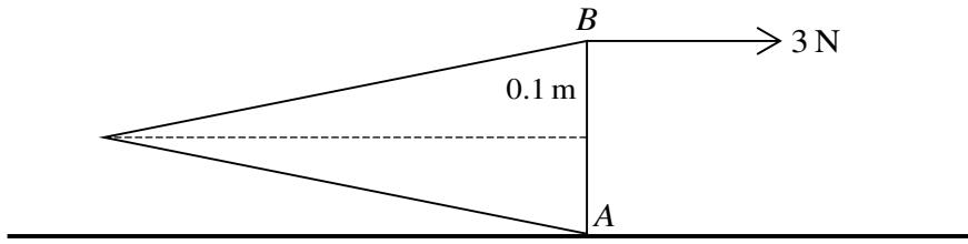
A uniform solid cone has weight 5 N and base radius 0.1 m.  $AB$  is a diameter of the base of the cone. The cone is held in equilibrium, with  $A$  in contact with a rough horizontal surface and  $AB$  vertical, by a force applied at  $B$ . This force has magnitude 3 N and acts parallel to the axis of the cone (see diagram). Calculate the height of the cone. [3]
