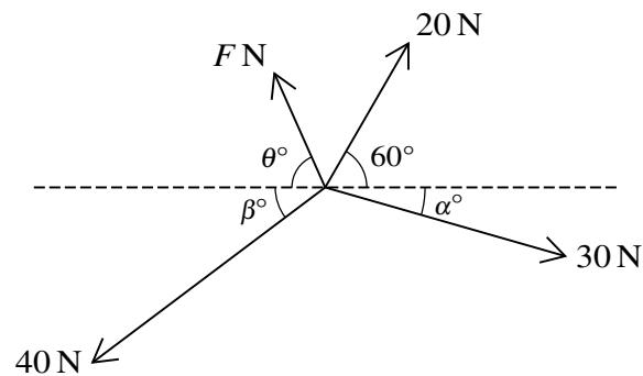
Four coplanar forces act at a point. The magnitudes of the forces are 20 N, 30 N, 40 N and  $F$  N. The directions of the forces are as shown in the diagram, where  $\sin \alpha^\circ = 0.28$  and  $\sin \beta^\circ = 0.6$ .
