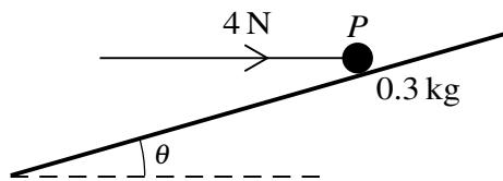
A particle  $P$  of mass 0.3 kg rests on a rough plane inclined at an angle  $\theta$  to the horizontal, where  $\sin \theta = \frac{7}{25}$ . A horizontal force of magnitude 4 N, acting in the vertical plane containing a line of greatest slope of the plane, is applied to  $P$  (see diagram). The particle is on the point of sliding up the plane.
