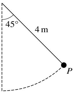
A child of mass 35 kg is swinging on a rope. The child is modelled as a particle  $P$  and the rope is modelled as a light inextensible string of length 4 m. Initially  $P$  is held at an angle of  $45^\circ$  to the vertical (see diagram).
