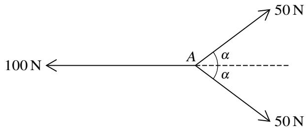
Three coplanar forces of magnitudes 100 N, 50 N and 50 N act at a point  $A$ , as shown in the diagram.
