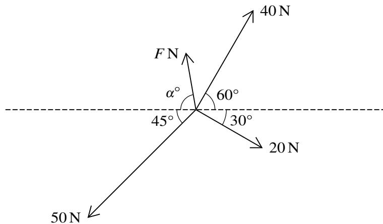
Four coplanar forces of magnitudes 40 N, 20 N, 50 N and  $F$  N act at a point in the directions shown in the diagram. The four forces are in equilibrium.
