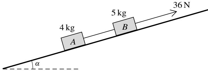
Two blocks  $A$  and  $B$  of masses 4 kg and 5 kg respectively are joined by a light inextensible string. The blocks rest on a smooth plane inclined at an angle  $\alpha$  to the horizontal, where  $\tan \alpha = \frac{7}{24}$ . The string is parallel to a line of greatest slope of the plane with  $B$  above  $A$ . A force of magnitude 36 N acts on  $B$ , parallel to a line of greatest slope of the plane (see diagram).
