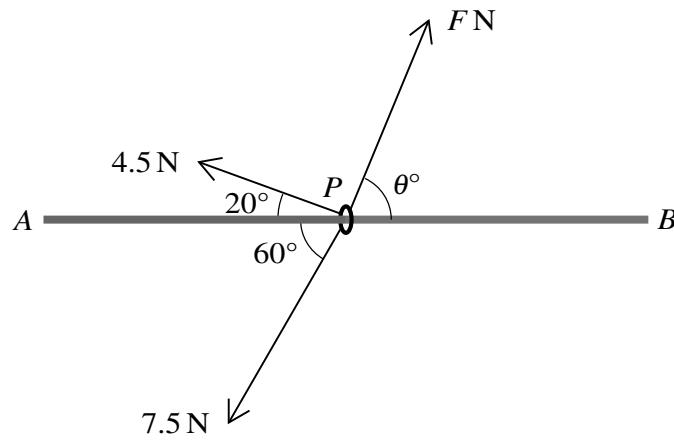
A small ring  $P$  is threaded on a fixed smooth horizontal rod  $AB$ . Three horizontal forces of magnitudes  $4.5\text{ N}$ ,  $7.5\text{ N}$  and  $F\text{ N}$  act on  $P$  (see diagram).
