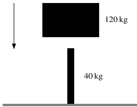
A metal post is driven vertically into the ground by dropping a heavy object onto it from above. The mass of the object is 120 kg and the mass of the post is 40 kg (see diagram). The object hits the post with speed  $8 \text{ m s}^{-1}$  and remains in contact with it after the impact.
