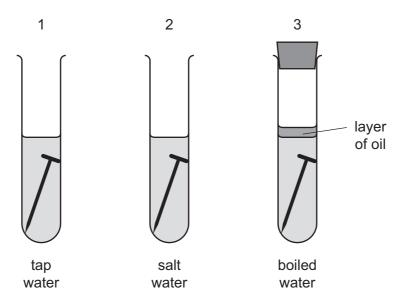
In which test-tubes do the nails rust?
